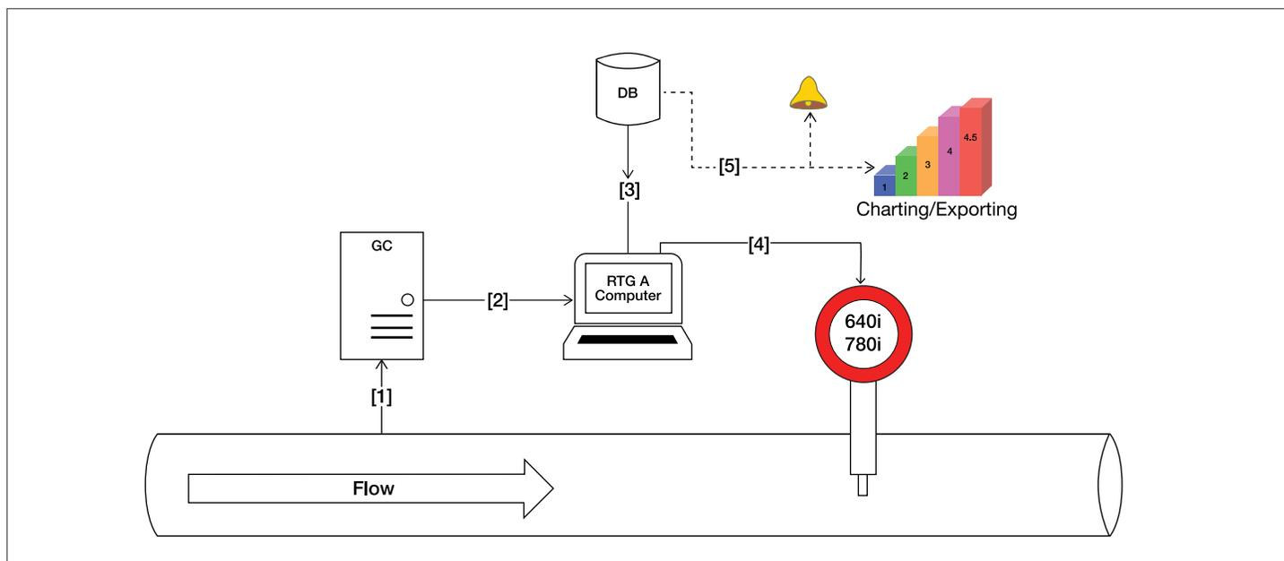
Figure 3. QuadraTherm® 640i/780i with qMix-RealTime™ app integrated with gas chromatograph
